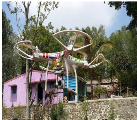
Fig 5.7.3.1.4 UAV used to spray the pesticides on infected coconut tree at Hosahalli, Tumkur.
