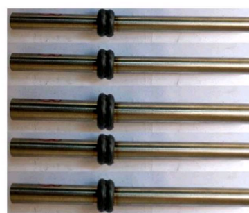
Fig 3: NiTiNol rods welded
