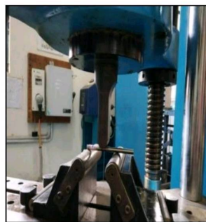
Fig 5 :Sample on bending test
